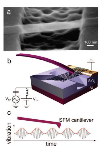
**Figure 1.** Device and experimental setup. (a) A scanning electron microscope image of a suspended graphene resonator. (b) Schematic of the resonator together with the SFM cantilever. (c) Motion of the suspended graphene sheet as a function of time. A high-frequency term at  $f_{\rm RF}$  is matched to the resonance frequency of the graphene, and the resulting oscillation is modulated at  $f_{\rm mod}$ .
