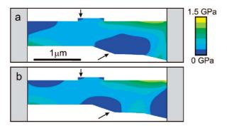
**Figure 4.** Calculated principal stress  $\sigma_1$  for the suspended graphene sheet in Figure 3. The color scale shows the stress in the resonator, ranging from 0 to 1.5 GPa. (a) Top surface. (b) Bottom surface. Arrows indicate regions with low stress where the amplitude of the eigenmodes is maximum.
